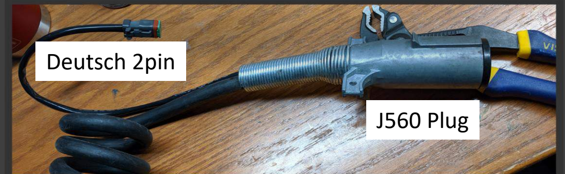
Custom Umbilical Cable Tap
