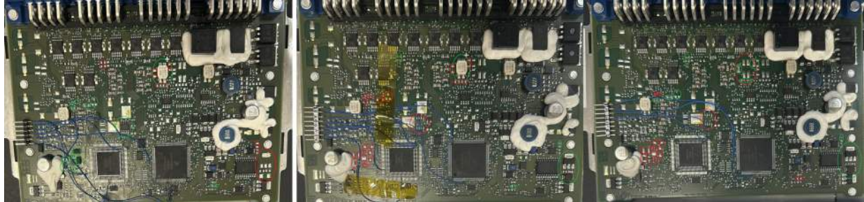
Figure 2: The PCBs of the three EC80s acquired and tested. A 0.1” header is installed for access to the BDM programming pins on the right S12X MCU. The added/removed components are highlighted in green/red, respectively.
