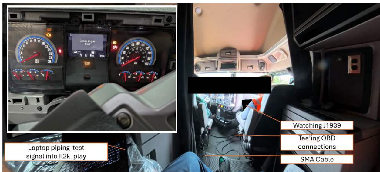
Figure 17: Top Left: failure state of instrument cluster after any and all the ECU crashes described in Section 8 while still in-motion. Wide: in-cab picture of in-motion vehicle test with black bar redacting.
