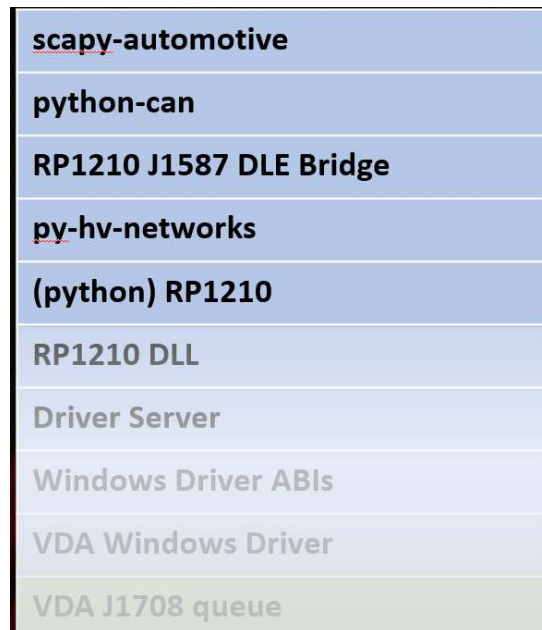
diagram of the python-can software stack enabled by the custom 'RP1210 J1587 DLE Bridge' developed.
