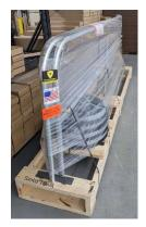
**Stowability—**When railings are tendered in boxes or crates, a flat load-bearing surface will generally be present, which would allow for other freight to be loaded on top of the handling unit. There will typically be lateral support for adjacent freight as well.
