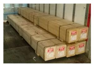
**Stowability**—Fittings and shorter lengths of pipe or tubing may be tendered in boxes, often unitized on lift truck skids or pallets, while longer pieces may be tendered in boxes, bundles or crates. When tendered in boxes or crates the shipments generally provide a flat load-bearing surface.
