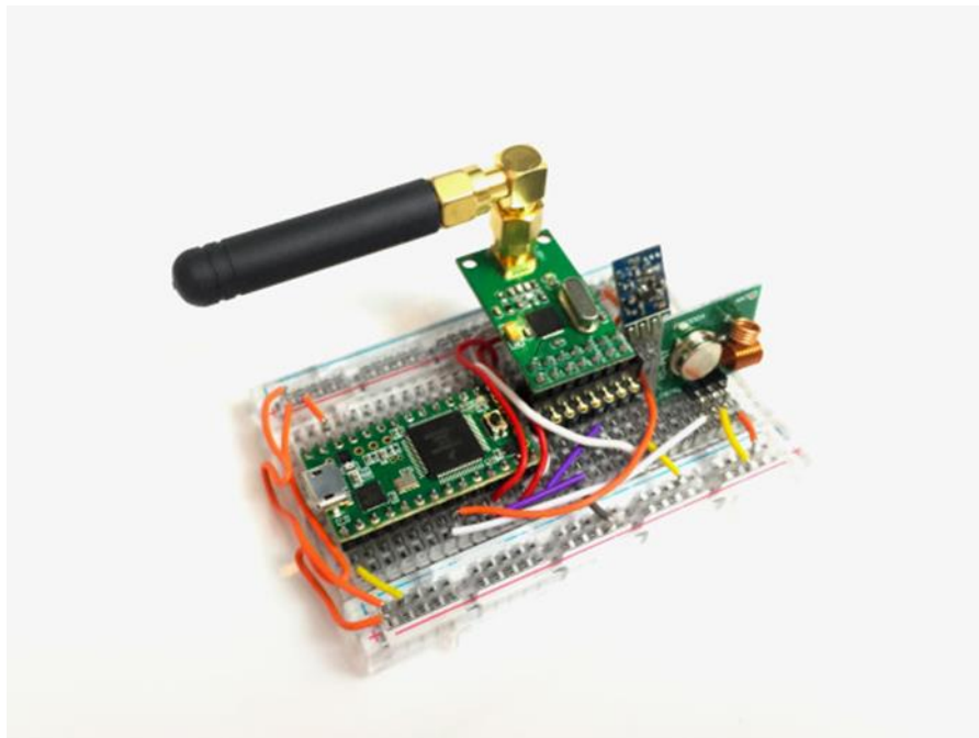
Figure 11 - RollJam Car Unlocking Device
