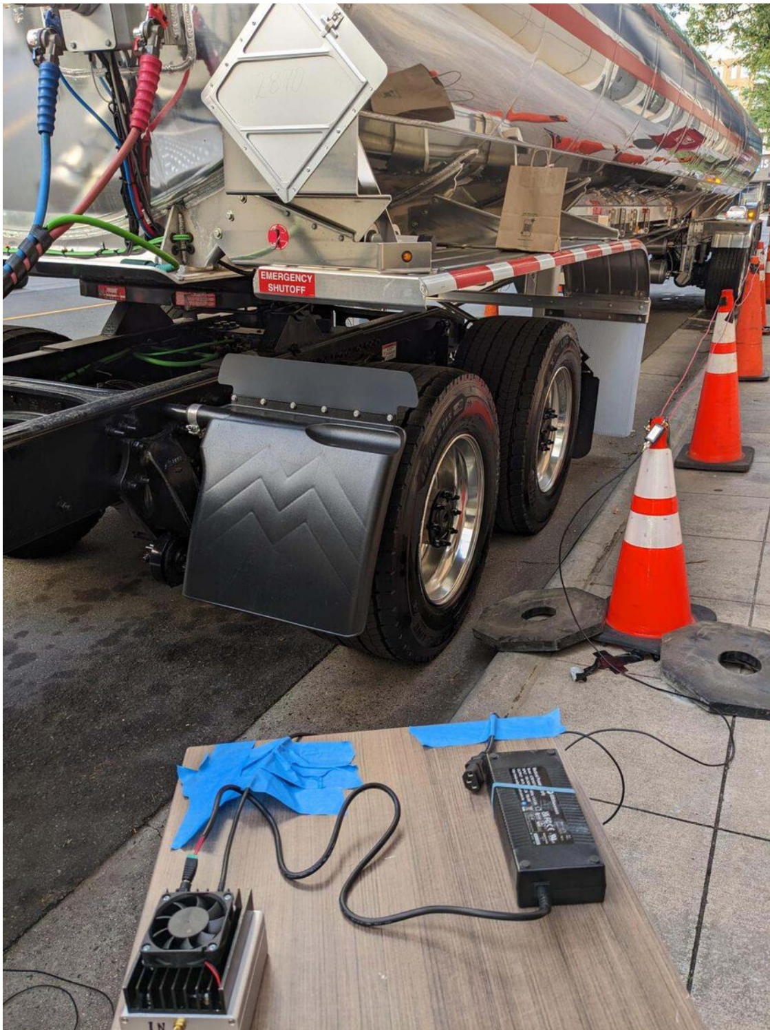
typical table location between tractor and trailer, also showing locations of (from left to right): 500W, 300USD, power amplifier, 48V power supply for amplifier (disconnected), RF SMA-SMA
